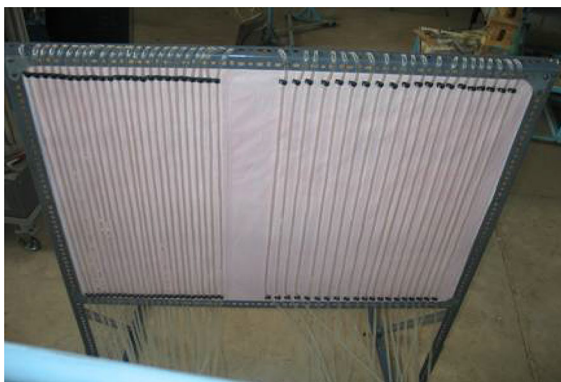
Fig. 6 Schematic of the board piezometers
